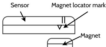
To reduce risk of damage over time, place the sensor on the frame and the magnet on the door or window itself.
