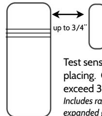
Test sensor before placing. Gap should not exceed 3/4".
