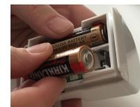
Insert batteries to place device in "learn" mode
