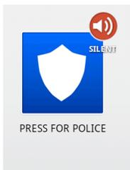
An "Intrusion" alarm is triggered when you touch the "Police" panic button. (touching "silent" triggers a silent alarm.) For your security, once a police siren has been triggered it cannot be silenced without a passcode.
