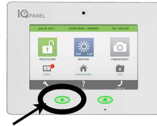
When you press the Emergency Button the Emergency Panic screen appears. Touching any of the buttons will trigger an alarm manually.
