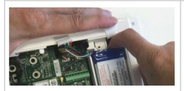
Use a finger or thumb and pull up firmly on the battery to remove.
