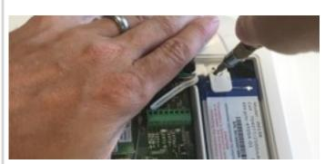
Remove the battery retaining clip and screw.
