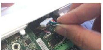
Remove retaining screw and back plate from the panel, then unplug the battery.
