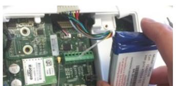
Place new battery into the battery slot (bottom first) pushing down into place. To ensure easier battery replacement in the future, do NOT use adhesive tape. Screw down retaining bracket, plug in battery and replace panel back plate.
