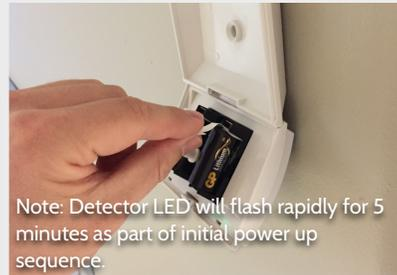
Note: Detector LED will flash rapidly for 5 minutes as part of initial power up sequence.
