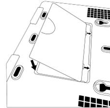
Replace the cover by inserting the top first, then while making sure the cable passes under the opening firmly press down on the bottom until the cover “snaps” into place.
