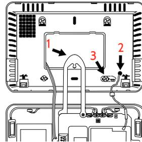
1. Hang the front of the panel with the hanging strap on the back plate as shown above.
