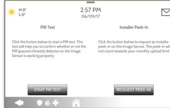
**PIR Test** checks the motion sensor
