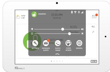
To access the Advanced Settings menu pull down the Settings tray at the top of the screen, select “Settings” and then “Advanced Settings”. Enter your dealer, installer or master code. The code used to enter Advanced Settings determines the level of access. When using partitions the code entered at the screen lock determines the access level for Advanced Settings.
