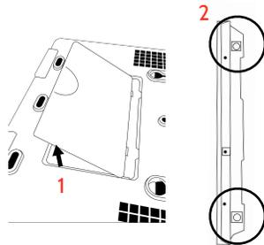
1. Insert your thumb or finger under the opening on the back cover and firmly pull up to remove. This cover is not needed for wall mount.
