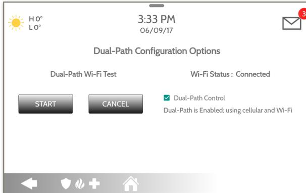
By default Dual-Path Control is enabled. To disable, “un-check” the box.
