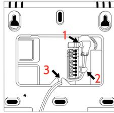
1. With the included power supply and cable, plug the barrel connector into the jack next to the terminals as shown above.
