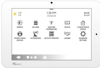
The Settings page allows quick access to various simple features & settings that do not require the protection of a Dealer, Installer or Master code to be changed.
