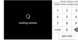
If using S2 Authenticated, enter the first 5 digits of the DSK or scan the QR Code from the box
