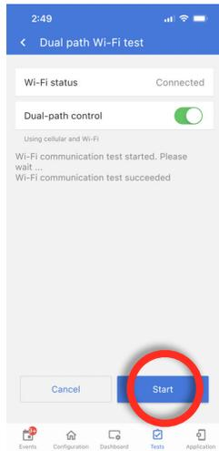
By default Dual-Path Control is enabled. To disable, “toggle” the Dual-path control slider off.
