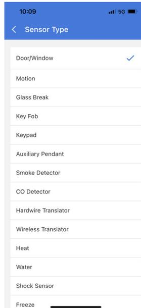
**Note:** for UL/cUL, only UL/cUL listed devices shall be used: Door/Window contact: 60-362N-10-319.5, Motion Detector: 60-639-95R, Smoke Detector: IQ Smoke QS5110-840. For UL2610 installations use only UL listed PowerG devices.
