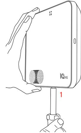
1. With a small phillips screwdriver, screw in the locking screw from the bottom of the panel to secure it to the wall.
