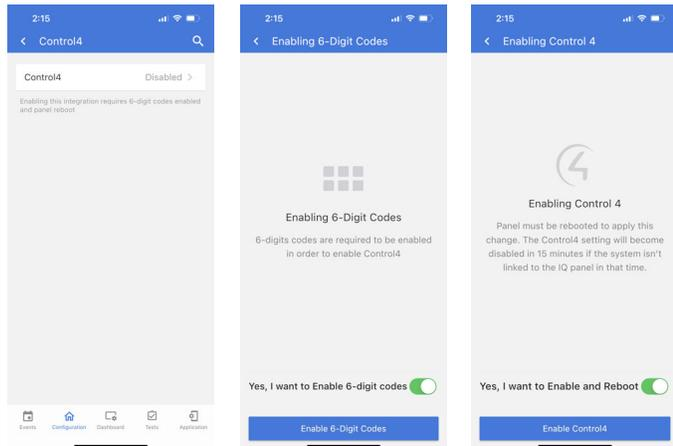
Prior to enabling Control4 integration you must enable 6-digit user codes.
