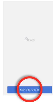
Press “Start Clear Device” then press the “Pair” or “Learn” button on device
