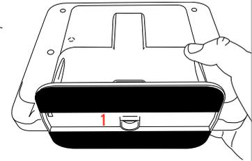
1. With a small Phillips screwdriver, screw in the locking screw from the bottom of the panel to secure it to the table stand.
