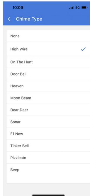
Because of the dynamic nature of the way the IQ4 NS pairs and understands each individual sensor, you can program each sensor to have a unique chime or even turn chiming off for that individual sensor. To customize your chime for a particular sensor touch the Chime Type drop down and choose from the list.
