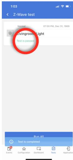
To perform a Z-Wave Test, touch the “Run All” button. A successful test will result in a “Pass” and a time stamp.
