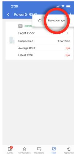
Average and Latest RSSI values are automatically stored as sensors communicate over time. This helps give a picture of how well a sensor is communicating with the panel.
