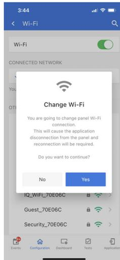
Touch “Wi-Fi” under the configuration tab, then select a network from the list to connect to. Type in the password (encryption key) to connect.
