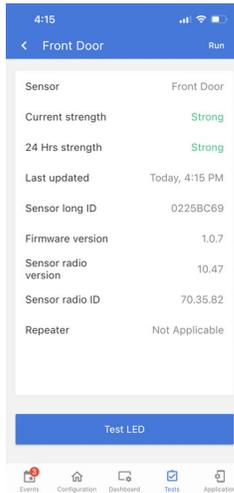
Touch “Run” to query the signal strength from the sensor.
