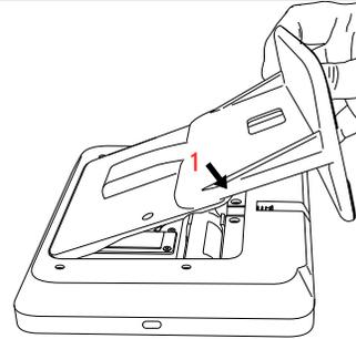
1. Locate the SmartMount table stand and insert the hooks into the back of the panel, then swing down and press into place.
