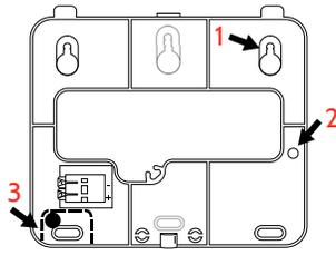
1. Mount the backplate to the wall using flat head screws\* and appropriate wall anchors if needed, ensuring it is level.
