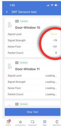
The Sensor Test shows a summary page of each sensor paired to the panel along with the last event's dBm level, noise floor and how many packets were received from the sensor.
