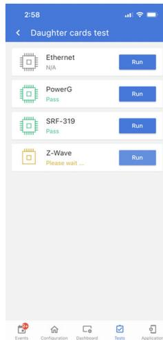
Select “Run” on an individual available card to start the test. In some cases the test may take several minutes after which the panel will show a result of a “Pass” or “Fail”.
