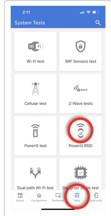
\*PowerG daughter card must be installed in the panel to access this test.
