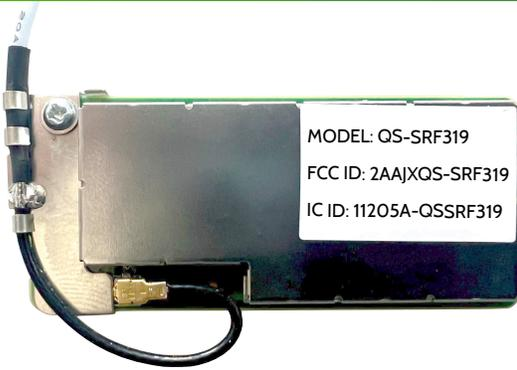
The IQ Card-319 can be installed in to “Slot 3” of your IQ Panel 4, IQ4 Hub or IQ4 NS to enable support of approved S-Line & legacy 319.5 MHz SRF sensors.
