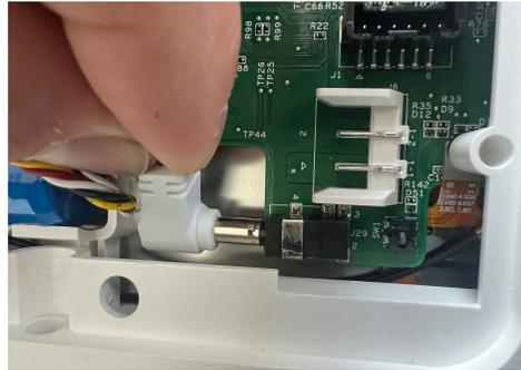
Once the IQ Panel has completely powered down, unplug or disconnect the power by removing the barrel jack connector inside the panel or by unplugging the power supply. **NOTE: it is NOT required to disconnect the battery.**
