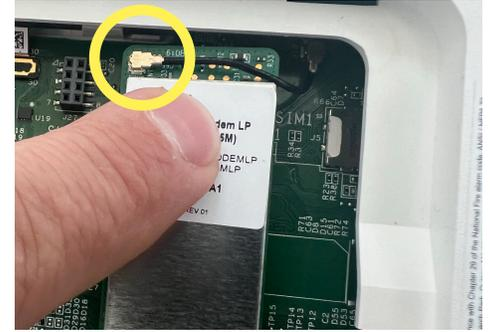
Push the IQ Card firmly into place. Connect the PowerG antenna jumper to the daughter card.
