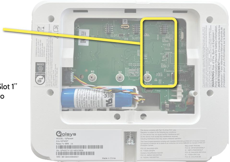
The IQ Card-PG can be installed in to “Slot 1” of your IQ Panel 4, IQ4 Hub or IQ4 NS to enable support of PowerG sensors.
