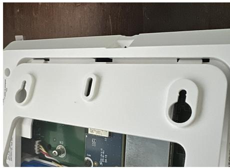
Replace the back cover, top tabs first. Press down on the bottom and tighten the retaining screw.
