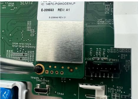
Install and tighten the provided locking screw to secure the IQ Card into place.
