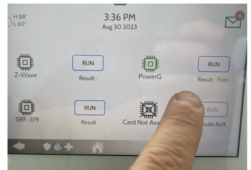
Run the "PowerG" test. Allow up to 2 min for the panel to successfully test the radio in the new IQ Card. If test fails, reboot the panel and try again.
