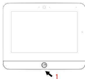
1. With a small phillips screwdriver, screw in the locking screw from the bottom of the panel to secure it to the wall.
