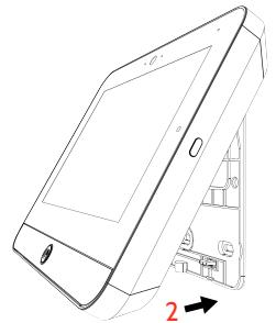
1. Latch the top of the IQ Panel 5 onto the SmartMount backplate
