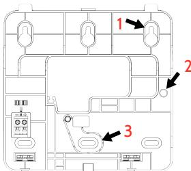
1. Mount the backplate to the wall using #6 flat head screws and appropriate wall anchors if needed, ensuring it is level.
