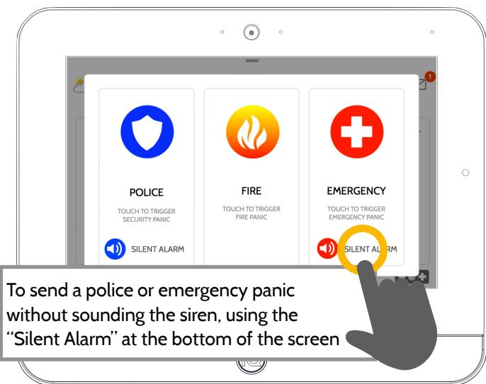
To send a police or emergency panic without sounding the siren, using the "Silent Alarm" at the bottom of the screen
