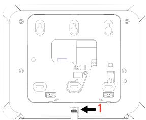
1. With a small phillips screwdriver, undo the locking screw from the back of the panel, remove the SmartMount backplate.
